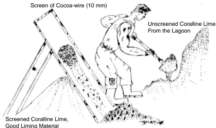
Figure 2. Screening coralline lime from the lagoon.
