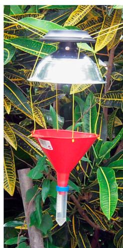
**Figure 1.** Light trap design. From top: solar light source (taken from landscape lights), aluminum reflector, plastic funnel, and removable centrifuge tube (made by coring and gluing the cap to the funnel tip).
