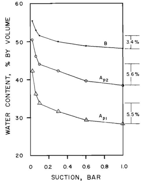
Fig. 2. Water-retention curves for a Haiku clay.
