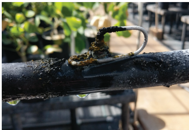
Figure 3. Example of a dirty irrigation head. The algal and mineral growth on this equipment can harbor disease and decrease the efficiency of the irrigation.
