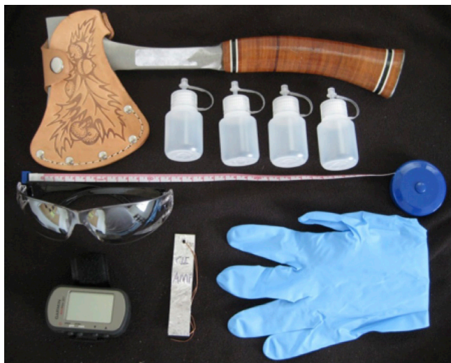
Figure 1. Equipment needed for installing an IPA trial, starting from the top: hatchet, liquid droppers, tape measure, PPE glasses, GPS, label tag, PPE gloves.
