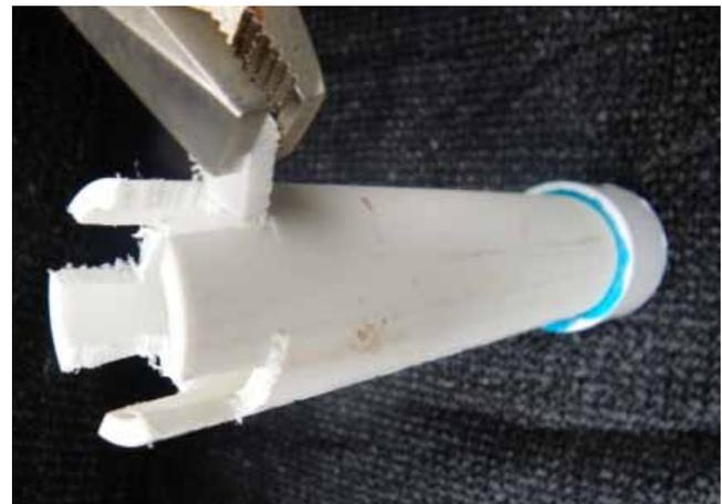
9. Remove the spacers between the teeth with pliers. If cut properly, the spacers break off cleanly with ease.
