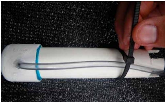
**14.** Tie the snorkel tube to bell pipe (above) and trim it (below). The bottom end of the snorkel tube should be above the teeth to ensure that air bubbles enter the bell siphon at the right time.
