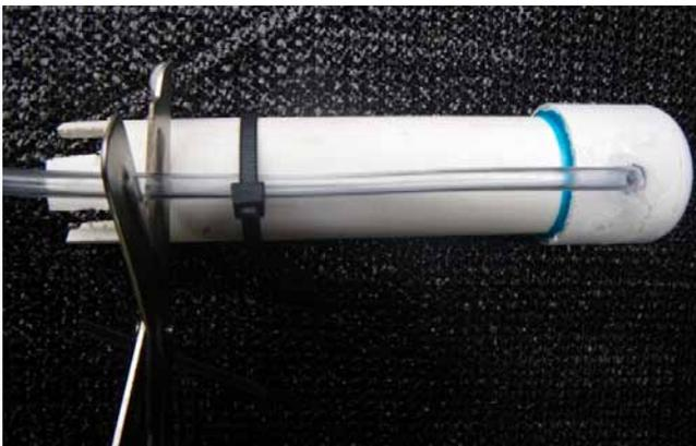
snorkel of the bell siphon. Gravel guards can be built in various ways, the simplest being with straight PVC pipe with holes or slits drilled or cut along its length to promote unrestricted water flow. Gravel guards should be approximately twice the diameter of the bell siphon, so that the bell siphon with its protruding snorkel can easily be moved on and off the standpipe during normal system operation and maintenance. Gravel guards should also be
