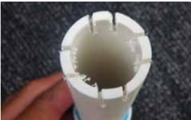
7. Notches, before the spacers between the teeth are removed.
