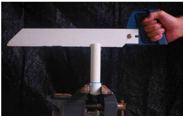
6. Cut notches to make teeth on the bottom of a bell tube. This can be done with various tools and methods.
