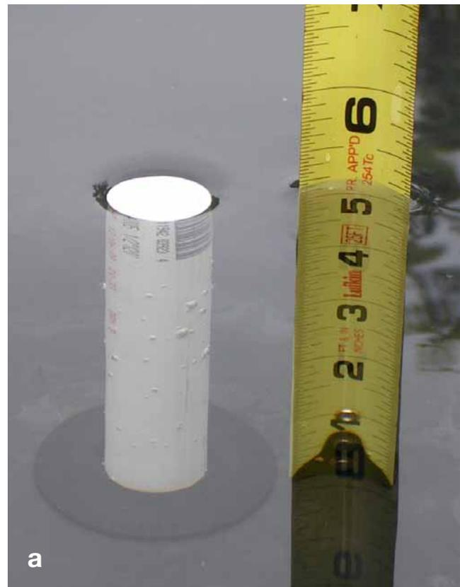
3a. The standpipe height determines the maximum depth of water in the grow-bed.
