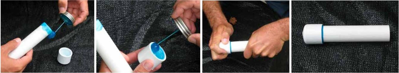
5. Attach the bell cap to the bell pipe with PVC primer and glue. After priming the inside surface of the cap and the outside surface of the pipe, apply glue to the rim of the pipe and the inside of the cap, as shown. Then, push the cap onto the pipe and twist the cap a quarter turn to seal the joint. Make sure the seal connecting the cap to the bell tube is airtight.
