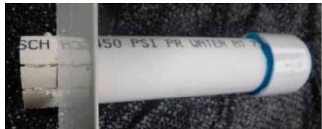
8. Make lateral cuts to weaken the spacers between the teeth.
