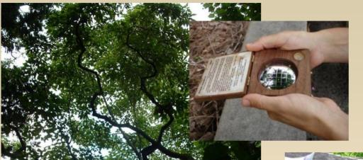
Spherical densiometer used to estimate forest canopy cover per plot
