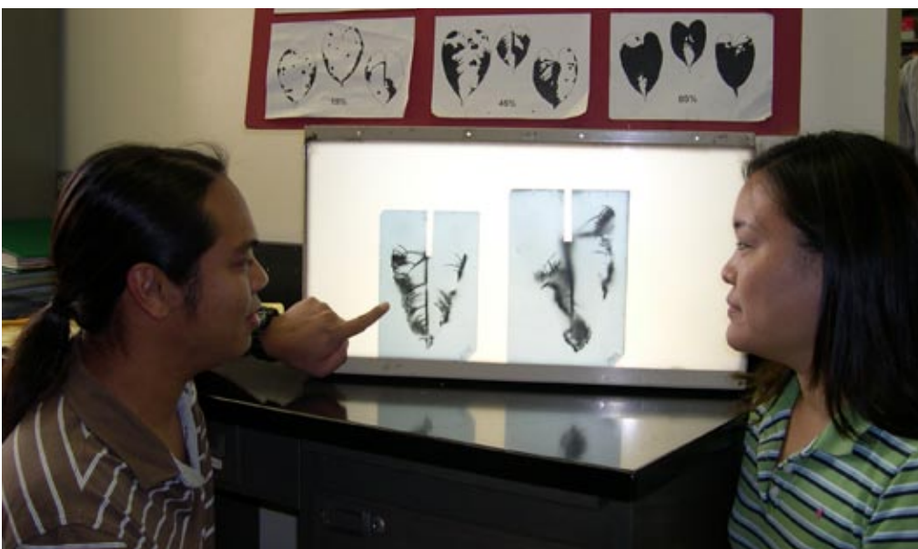
Peter and Tomie examining autophotographs produced by exposing X-ray film to a bioengineered bioluminescent strain of the bacterial blight pathogen. Colonization of the plant tissues is evident as black areas on the X-ray film even when no visible symptoms are present on the latently infected leaves.
