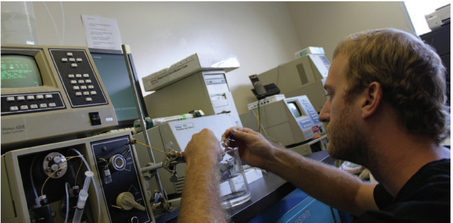
Mr. Zachary Bergeron conducting High Pressure Liquid Chromatographic separation of a synthetic cone shell toxin peptide, an analytical process commonly used in our development of novel pesticides.
