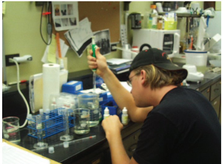
Aquaculture Laboratory (AnSci 465L) student, Austin Stankus, determines Ammonia, Nitrite, Nitrate, and pH levels in aquaponics and closed recirculation system water as part of class activities on materials balance.
