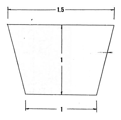
Volume is estimated using the assumption that the ratios of the (top diameter: bottom diameter: height) of a typical planting container are (1.5: 1.0: 1.0). Expressing the top and bottom radii, i.e., half the diameters, as a function of the container height and using the equation:
