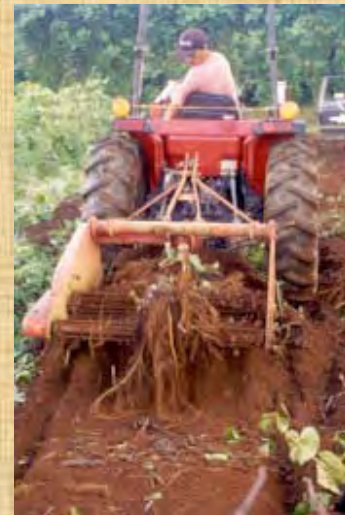
Modified sweet potato harvester, multiple plants
