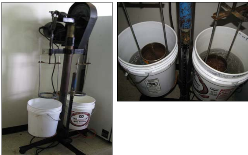
Picture 3.7. Mechanical oscillating sieving for measuring 1-2 mm stable soil aggregate; 30 oscillations per minute for 3 minutes sieving
