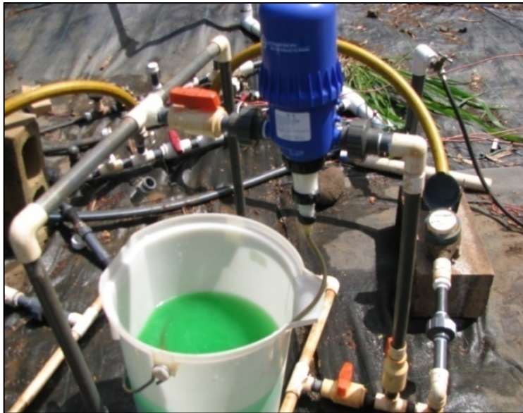
Picture 2.5. Injection fertilizer 90 kg N/ha as 19-19-19 within the drip irrigation Dosatron International DI 16 injection
