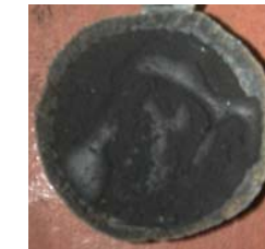
Figure 16. Water repellency in high VM charcoal (22.5%)
