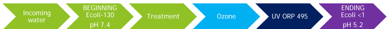
Scenario #5: Ozone treated with 2 in line filters (120-175 micron) FIRST then UV treatment
