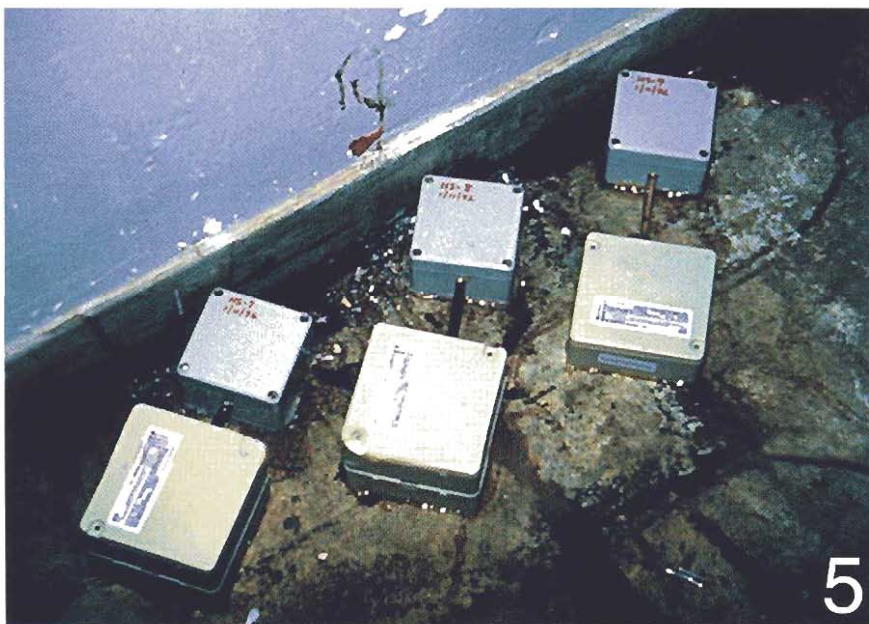
Fig. 5. Active prototype bait stations (along wall) connected to new prototype bait stations with 0.63cm tygon tubing.
