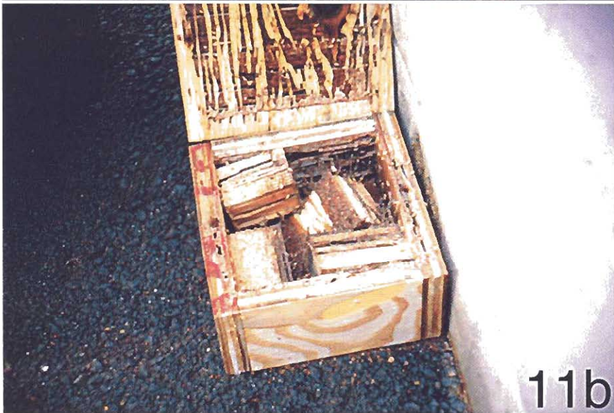
Fig. 11. a, Formosan subterranean termites were aggregated in wooden boxes placed along a cold joint; b, aggregated termites within a wooden box just prior to baiting.
