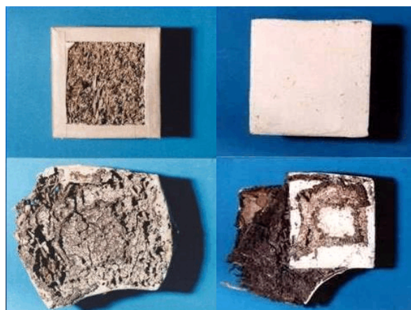
FIGURE 1. Compressed bagasse panels before (top) and after (bottom) exposure to Formosan subterranean termites in the field for four weeks. Note swelling of fibers due to moisture sorption.
