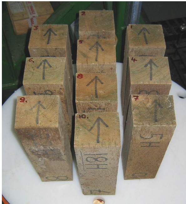
Figure 2 Dodai from Hawaii on CT scanner turntable
