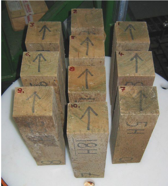
Figure 2 Dodai from Hawaii on CT scanner turntable
