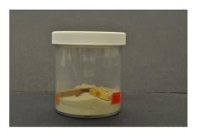
Figure 1. Sample test jar with three different wood species.
