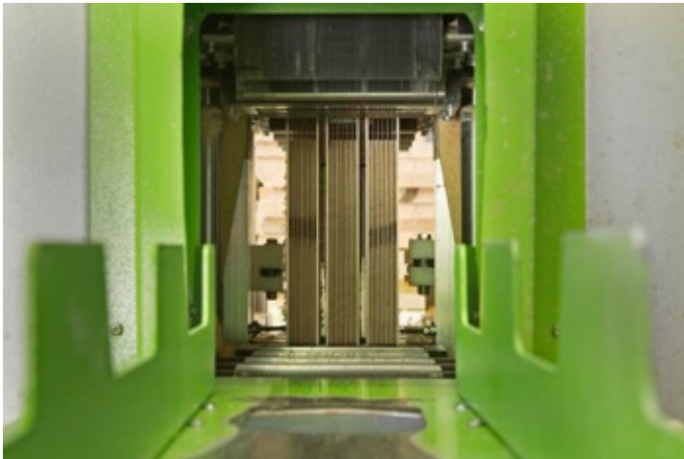
Figure 8: Frame saw making 18 pieces from 3.
