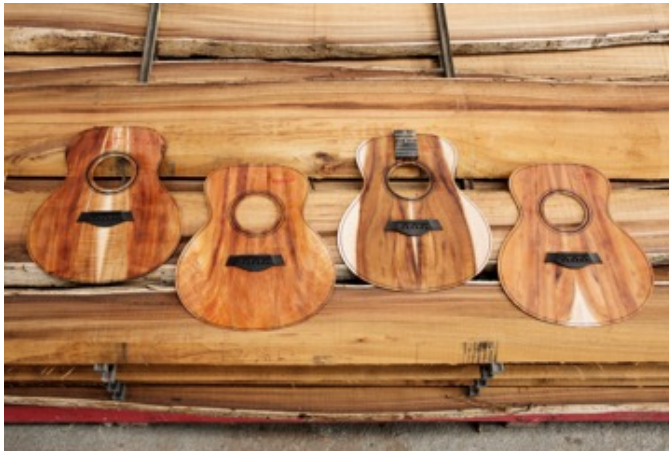
Figure 9: Taylor GS Mini Guitar tops glued up from 4 pieces.
