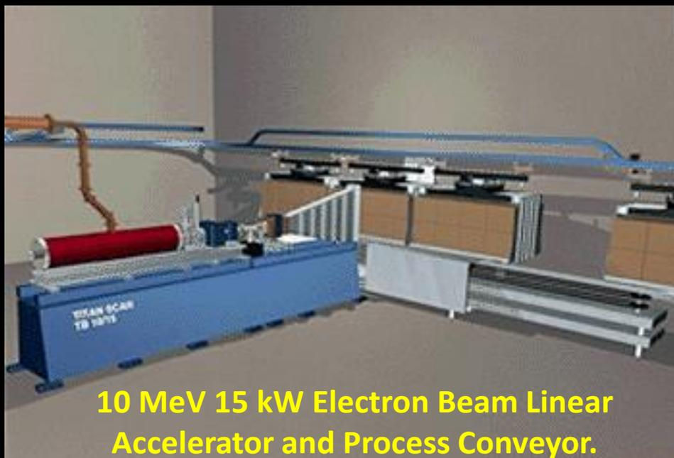
10 MeV 15 kW Electron Beam Linear Accelerator and Process Conveyor.
