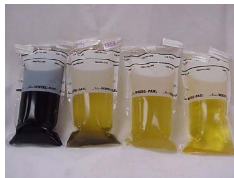
The two kits on the left (black and brownish) are positive. The two kits on the right (turbid and clear with light precipitate) are negative.
