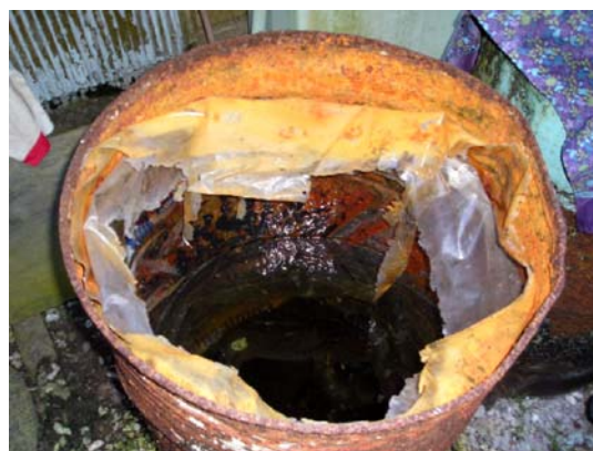
Metal drums, even when lined with thin plastic, do not make good catchments because bits of plastic, metal, and paint leach into the water.
