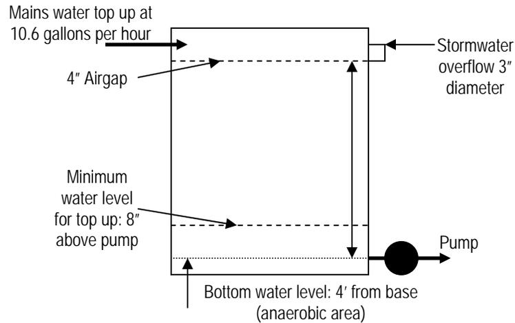
**Figure 3 – Rainwater Tank Configuration as used in PURRS**
