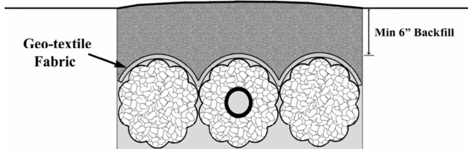
**Figure 7. Trench construction using polystyrene media.**
