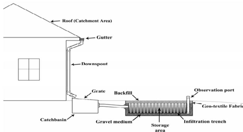
**Figure 1. Rainwater soil storage and infiltration system components.**
