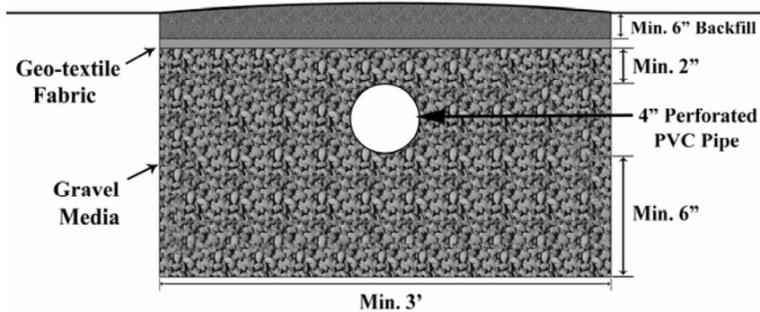
**Figure 5. Trench construction using a gravel media with perforated pipe.**
