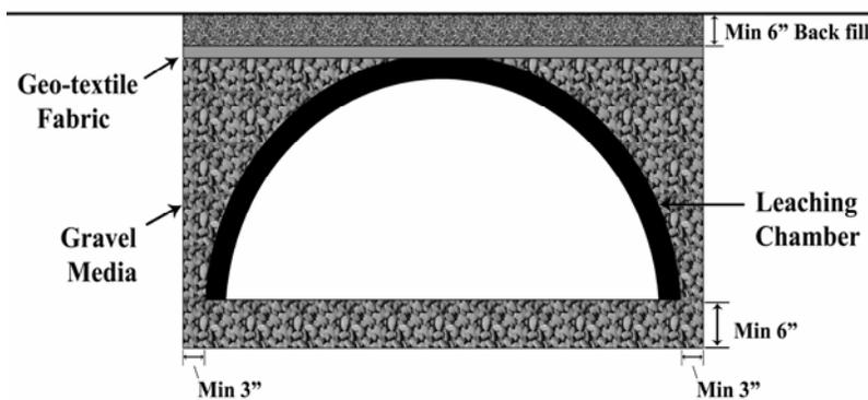
**Figure 6. Trench construction using a leaching chamber.**
