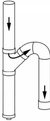
**Figure 4. Diagram of a “poor man’s” roof washer.**
