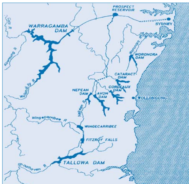
Figure 1. Sydney headworks system.
