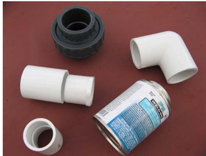
Sample plumbing fittings to attach your intake device (clockwise, from top): Union (allows you to access pipes again easily); 90-degree elbow; blue wet-or-dry plumbing glue; 1-inch coupler; 1/4-inch coupler next to threaded reducer bushing. Note: your system needs may vary.
