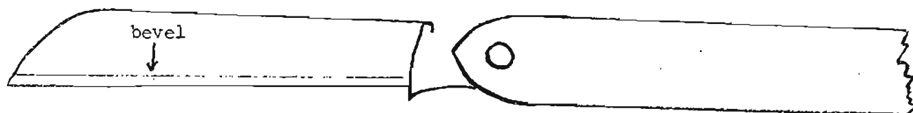
Figure 1. Grafting knife beveled for right-handed person.
