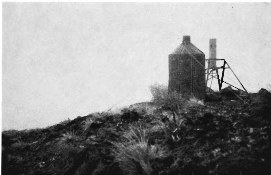
Figure 9. Raingauge of 900 inches capacity at summit of Waialeale. Much of the rain falls horizontally, being driven by strong winds coming over the cliff just beyond the gage. The gage is "unscreened."
