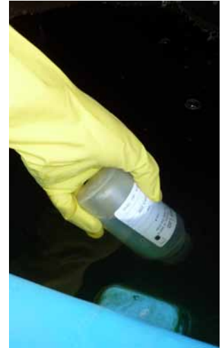
Take a water sample from the fish tank and have it tested for E. coli and other human pathogens.
