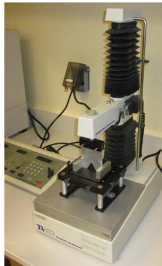
Figure 3. TA.XT2 texture analyzer fitted with a Warner-Bratzler blade used to measure shear force values of steak samples.
