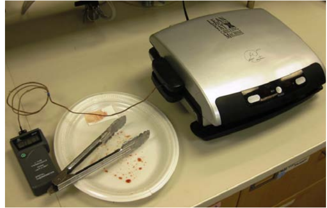
Figure 2. Ribeye steaks were grilled to reach a final internal temperature of 71°C (160°F) before being tested for shear force values.
