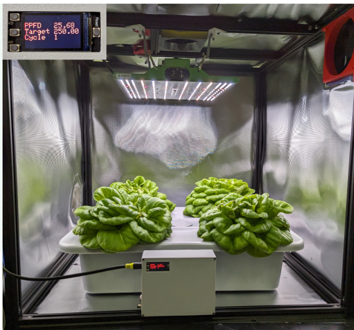
Custom controller adding supplemental LED light to hydroponically grown lettuce.
