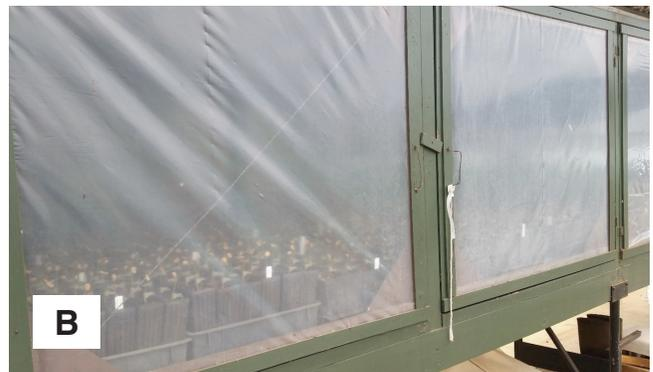
Figure 12b. Elevated humidity chamber.
