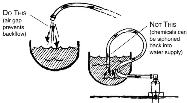
gap between the hose and the water in the pool. Toilets and washing machines have built-in air gaps.
