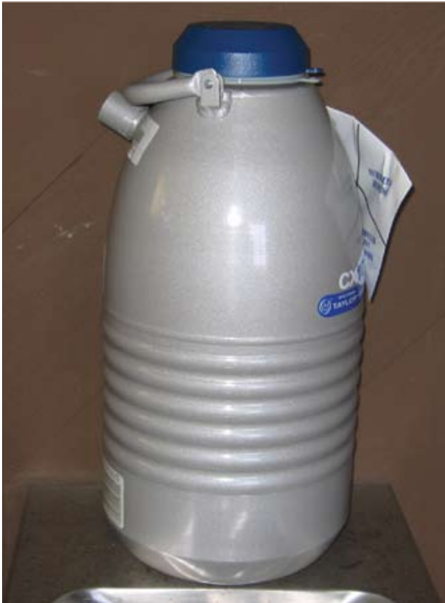
Figure 1. Liquid nitrogen tank.
