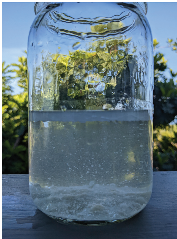
Figure 4. Jar Test showing coagulation of product, which indicates the tank mix will not be successful.
