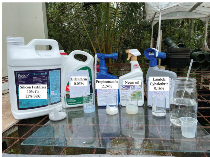
Figure 1. Jar Test set-up. Be sure to always begin the jar test with some water in the jar. Do not merely start mixing chemicals together in the jar without water.
