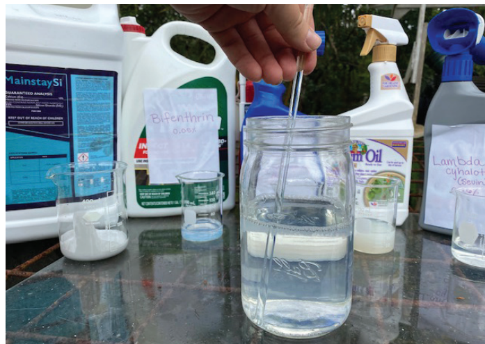
Figure 2. Jar Test mixing. Vigorously mix the ingredients with a clean plastic, glass, or metal stirrer to ensure the mix is homogenized.
