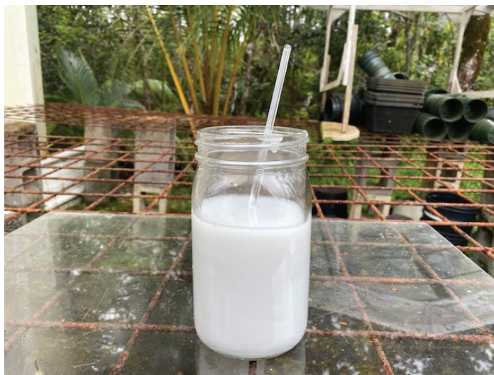
Figure 3. Completed successful Jar Test. No layering, precipitation, water gel, or coagulation is present.
