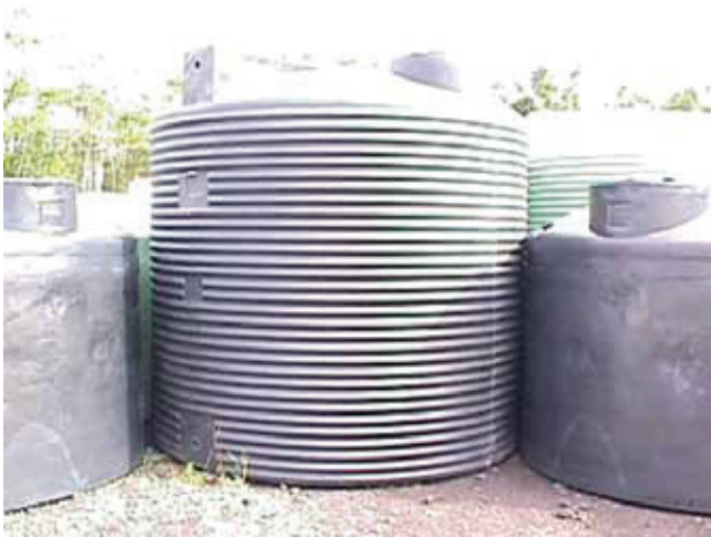
Polyethylene tanks are new to the market. They are lightweight, easy to relocate, and can be made out of food-grade materials. Their small size often requires joining multiple units to provide ample water storage. They can be molded with a solid cover.
