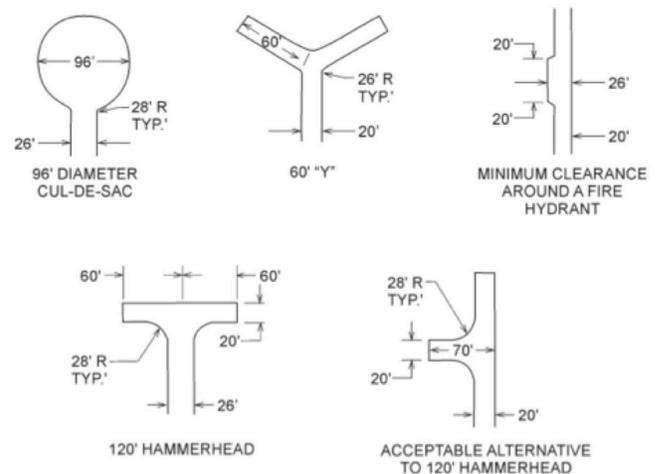
**Figure 6. Recommended turn-arounds for fire engines (by Oregon State [www.iccsafe.org/](http://www.iccsafe.org/)).**
