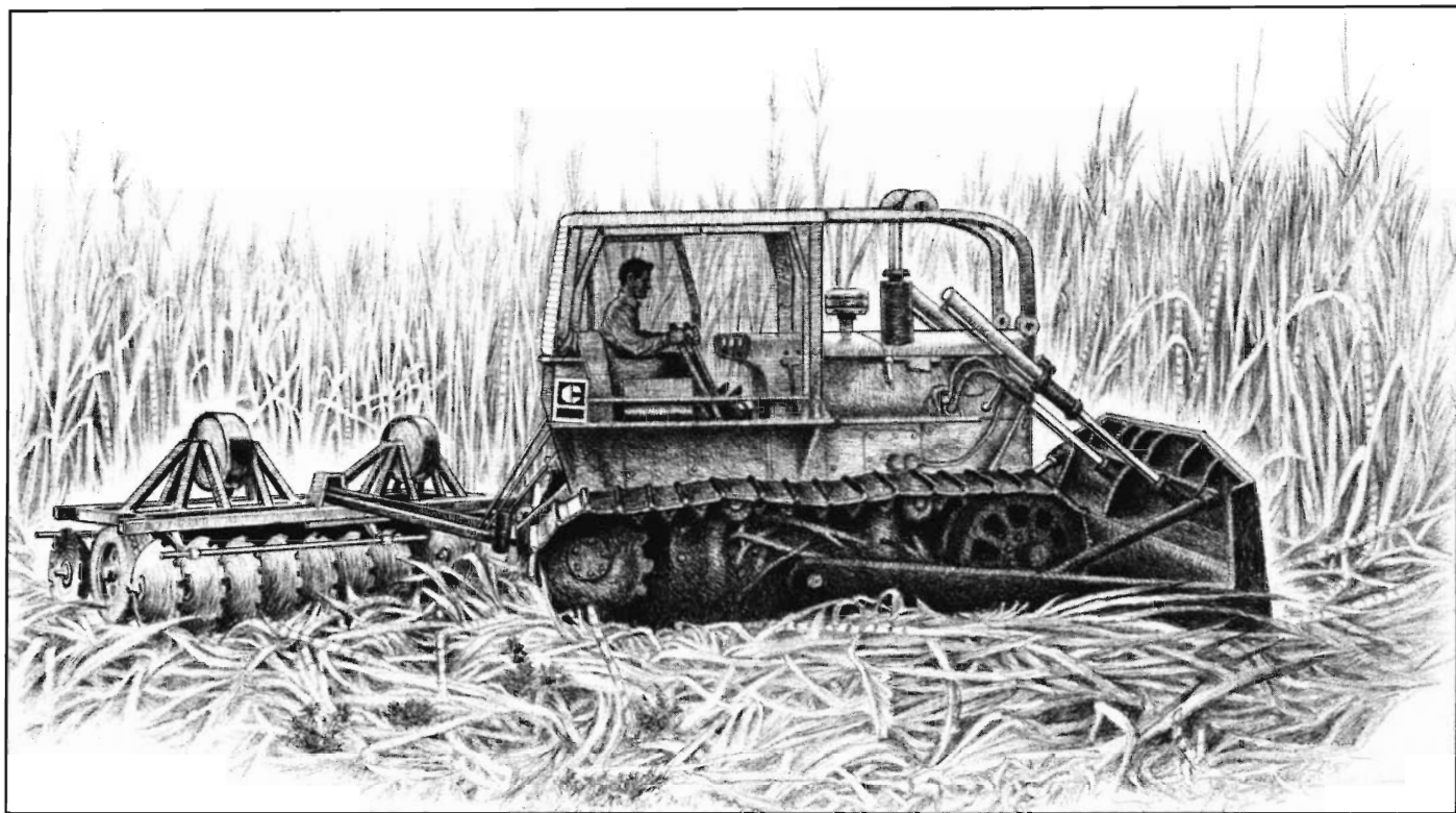
Figure 7 —D-6 tractor pulling cutaway harrow to clear abandoned candeland.
