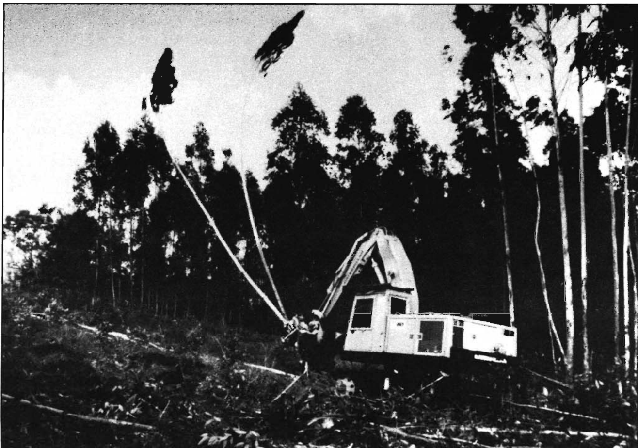
Figure 19—Harvesting using Caterpillar 227 fitted with feller-buncher head.
