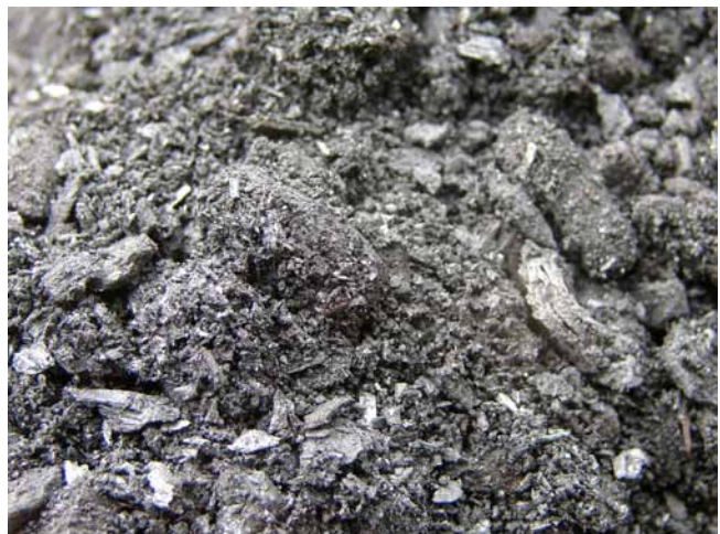
Production of biochar. Top, Melochia species logs (3–4 inches diameter) can serve as organic matter for biochar production. Center, biochar produced by heat treatment. Bottom, close-up of biochar particles; this material's size is called ½- ("half minus") because it consists of ½-inch or smaller particles.
