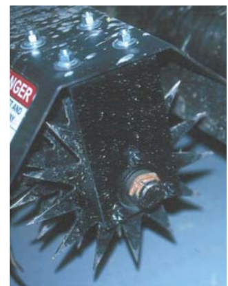
10. Spiking attachment for a power-driven reel mower (photo, A.S. McNitt)
