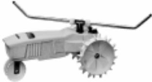
The **traveling** sprinkler usually has a whirling-type head and the traveling action can cover a large area without assistance. The path is guided by hose placement, which can easily be manipulated for large, irregular lawn shapes. Level ground and an overlapping pattern are required for even water distribution. This type is not suited for newly seeded lawns or other situations where soft soil conditions can lead to a stuck sprinkler.
