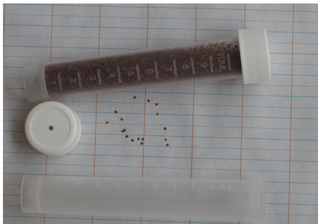
Figure 14. A shaker-type seeder may be fabricated from a test tube or small bottle with a \frac{5}{64} -in hole in the cap.
