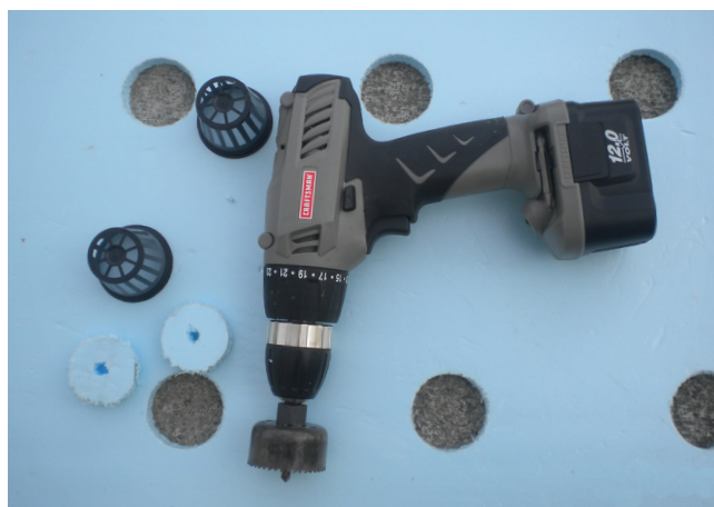
Figure 10. An electric drill with a 2-in hole saw is used to cut openings in the tank cover.
