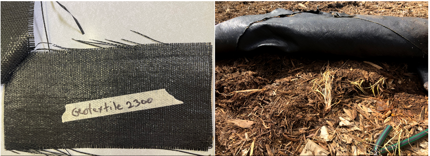
Figure 4. Polypropylene geotextile fabric-PGF used in the WC and MWCM plots. The PGF used in this study has the following specifications: trade name (Geotex 2300) distributor in Hawai'i (Rudy's Shade Inc.) manufacturer (Polyproductos), thickness (6.35 oz/sq yard), formulation (93.458% prime polypropylene, 4.85% black masterbach, 1.70% calcium carbonate).
