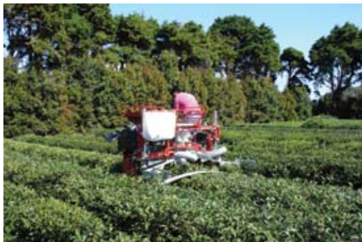
A pruning machine straddles a row for precision trimming and bush formation at Mealani.
