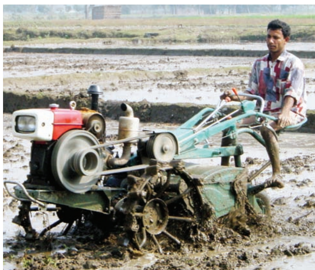
Figure 1. Wet-tilling (puddling) soil with a Chinese hand tractor. (Photo: P. Hobbs)
