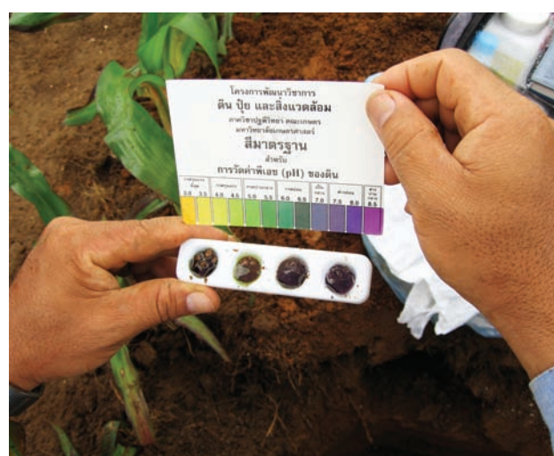
Figure 1. The Thai soil test kit was used not only in Laos (pictured here measuring pH 5.0), but also in West and Southern Africa.
