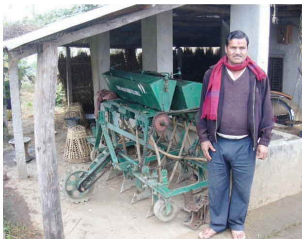
Figure 11. No-tillage drill introduced to two farmer groups in Nepal. (Photo: J. Duxbury)
