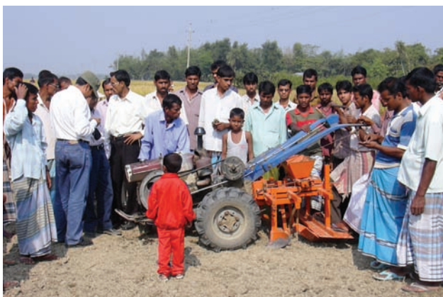
Figure 12. Bed planting attachment to Dong Feng Chinese hand tractor. (Photo: J. Duxbury)
