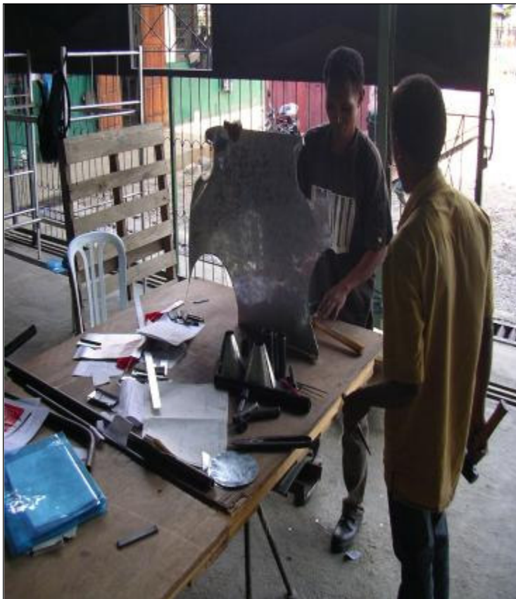
Trainees cut the metal plate for the 'cones' of the conical weeder
