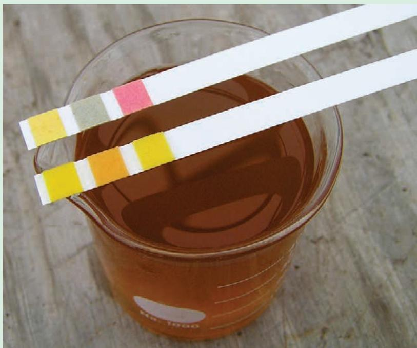
Tri-colored pH testing strips, before testing juice (above) and after testing (below). The colors after testing are compared with a master color chart to determine the pH value. PHOTO: S. NELSON
